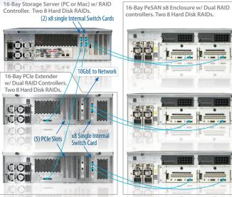
BlueStor PeSAN technology can be easily configured to handle the most complex workflow applications. Modular in design, BlueStor PeSAN can scale up to 4,100 TB using a combination of BlueStor sub-systems.
